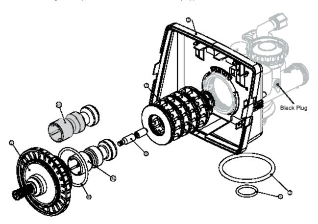
Drive Cap Assembly, Downflow Piston, Regenerant Piston and Spacer Stack Assembly
